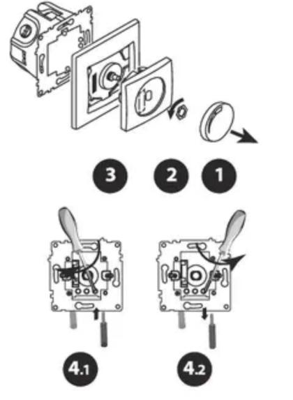
1. Remove the rotating button by pulling it upwards.
