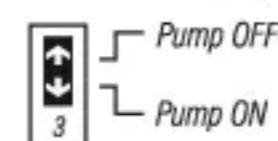
For hot water installations, it is recommended to activate the pump at least one minute every 24 hours in order to avoid seizure. Place switch #3 down to activate this function. For all other installations, leave switch #3 in the Off position (otherwise your system will be activated 1 minute every 24 hours).
