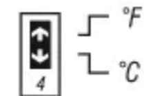
The thermostat is factory-set to °C. If you wish to change the temperature display to °F, slide switch #4 upward. Please note that if you change from °C to °F or vice versa, you must reset the Comfort (, Economy () and Vacation () settings accordingly.
