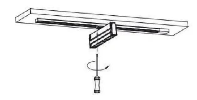
Step3.Adjust the position and angle of the track light.
